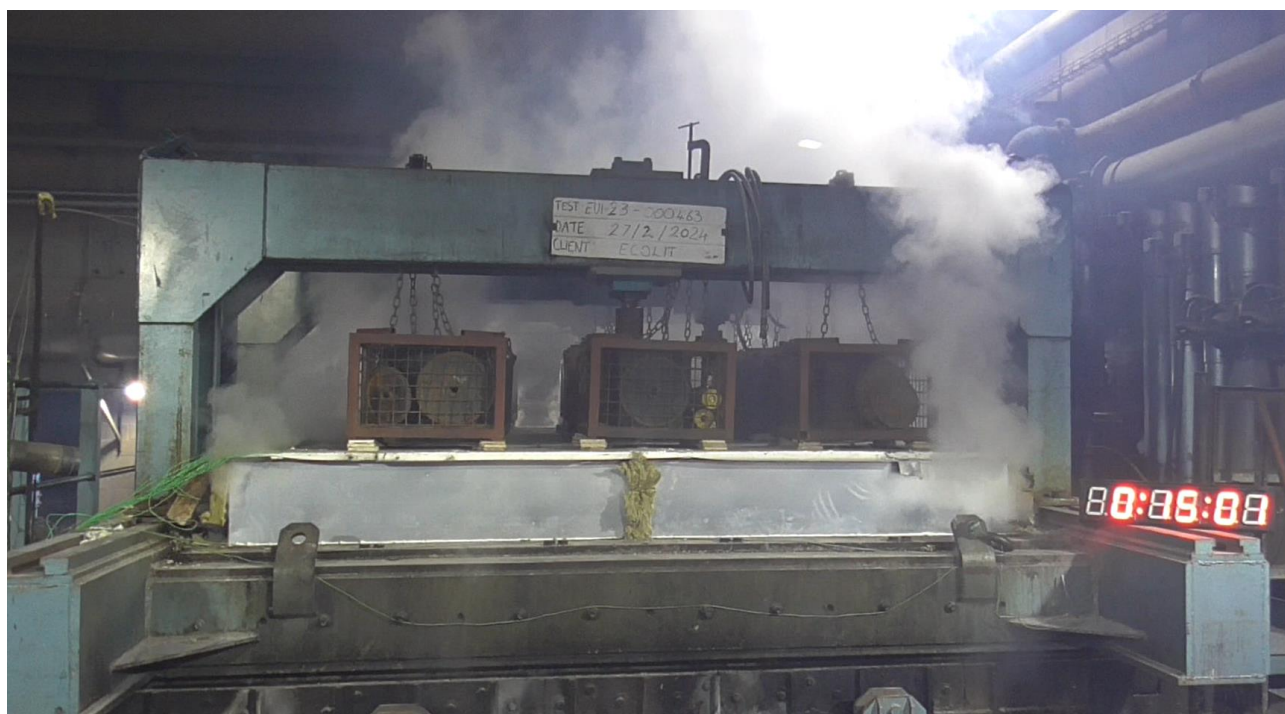
Photograph 9 - Detail of the unexposed side of the sample during the test. Photograph taken during minute 15.
