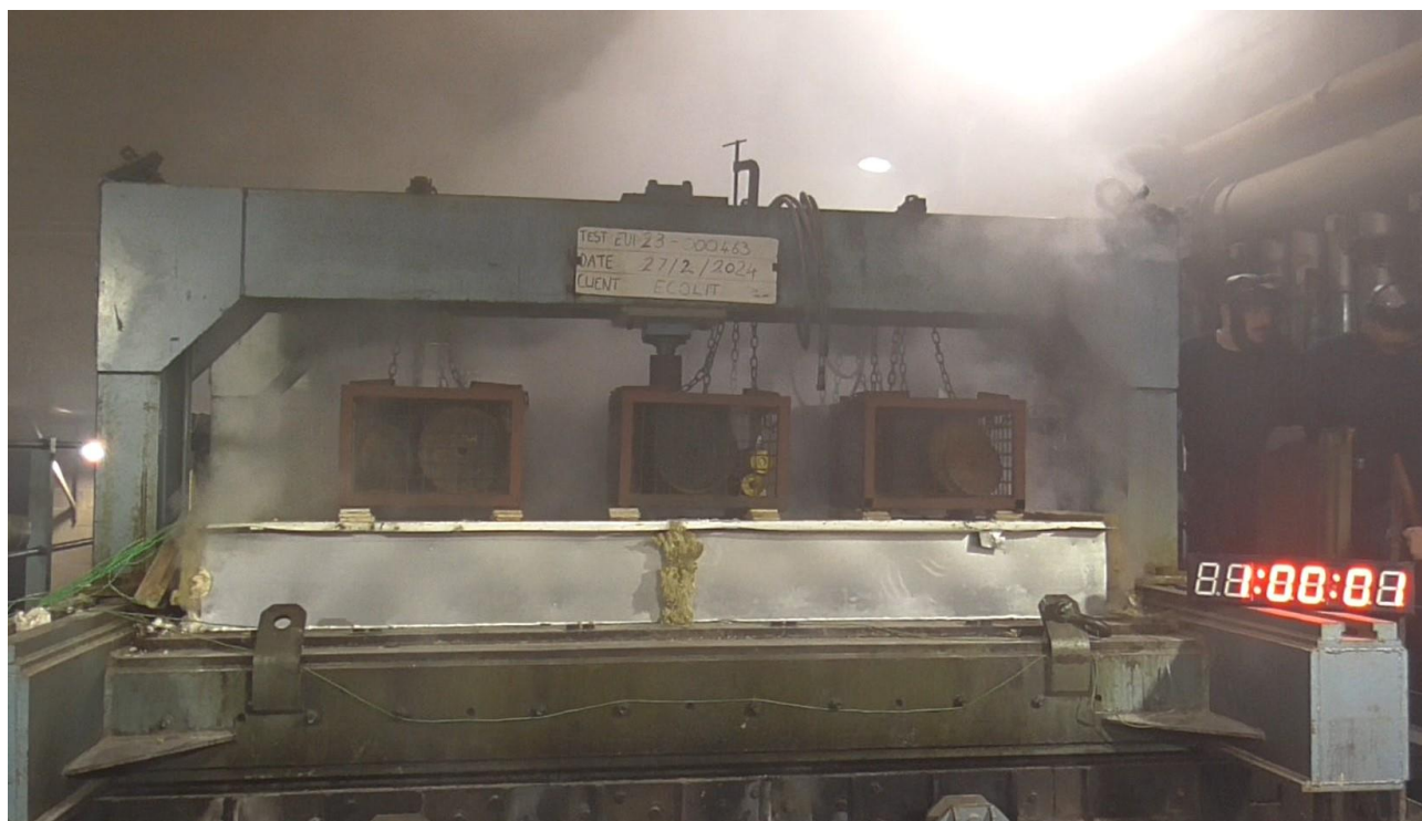
Photograph 16 - Detail of the unexposed side of the sample during the test. Photograph taken during minute 60.
