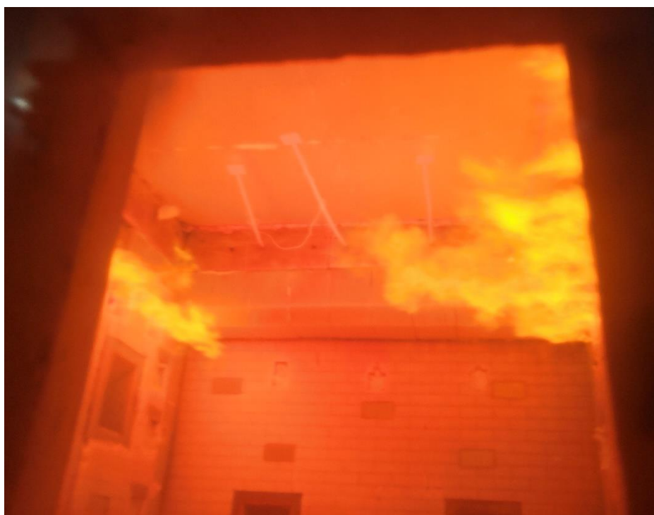
Photograph 15 - Detail of the exposed side of the sample during the test. Photograph taken during minute 57.
