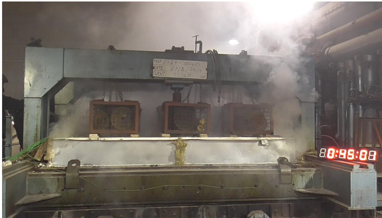
Photograph 14 - Detail of the unexposed side of the sample during the test. Photograph taken during minute 45.
