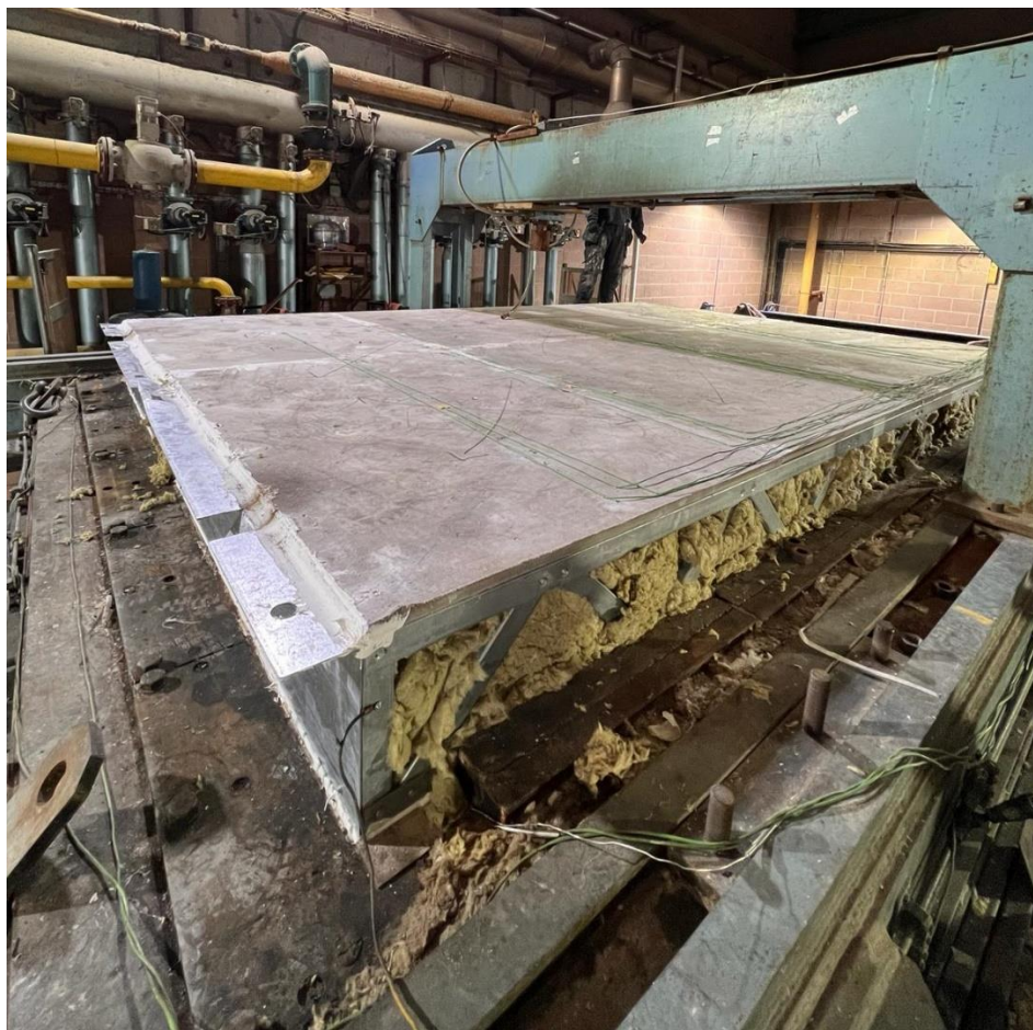
Photograph 4 - Detail of the unexposed side of the sample with side infill.
