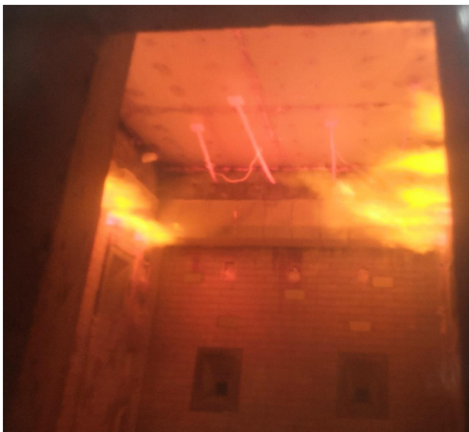
Photograph 10 - Detail of the exposed side of the sample during the test. Photograph taken during minute 25.
