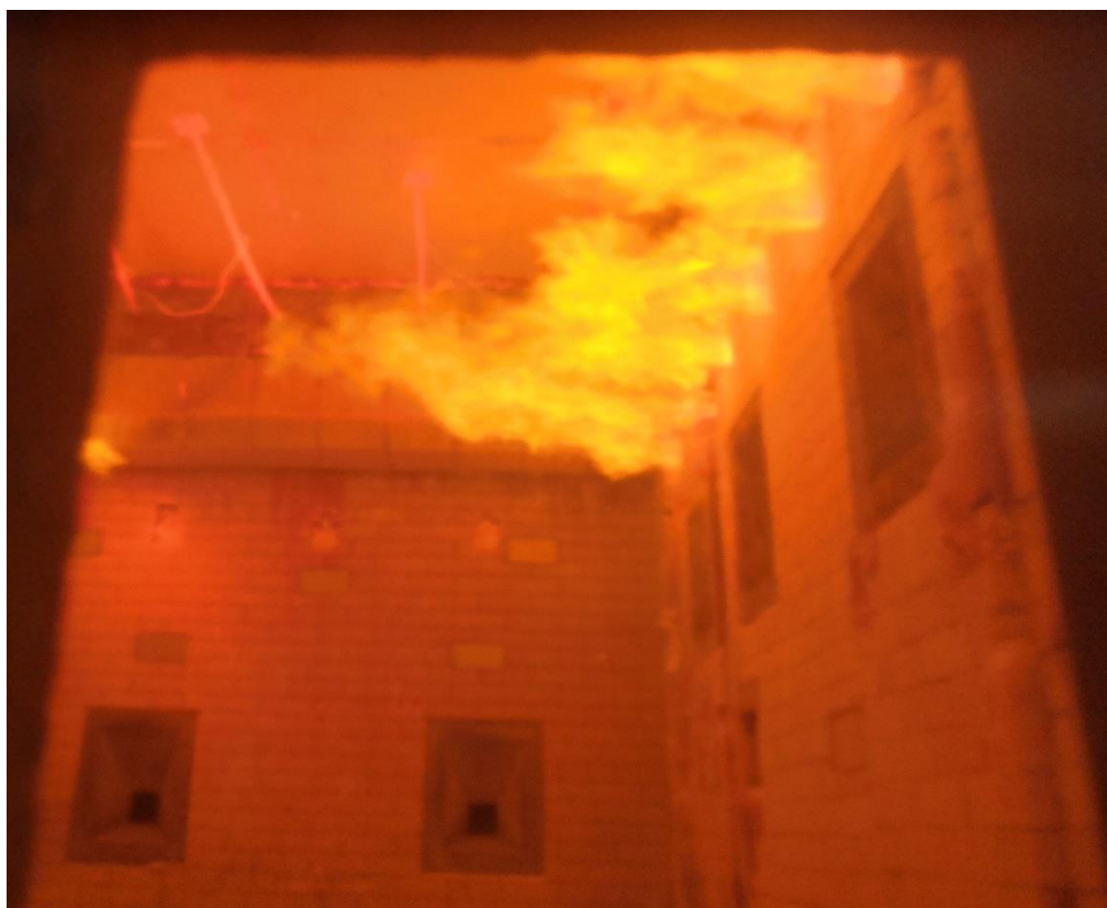
Photograph 12 - Detail of the exposed side of the sample during the test. Photograph taken during minute 35.
