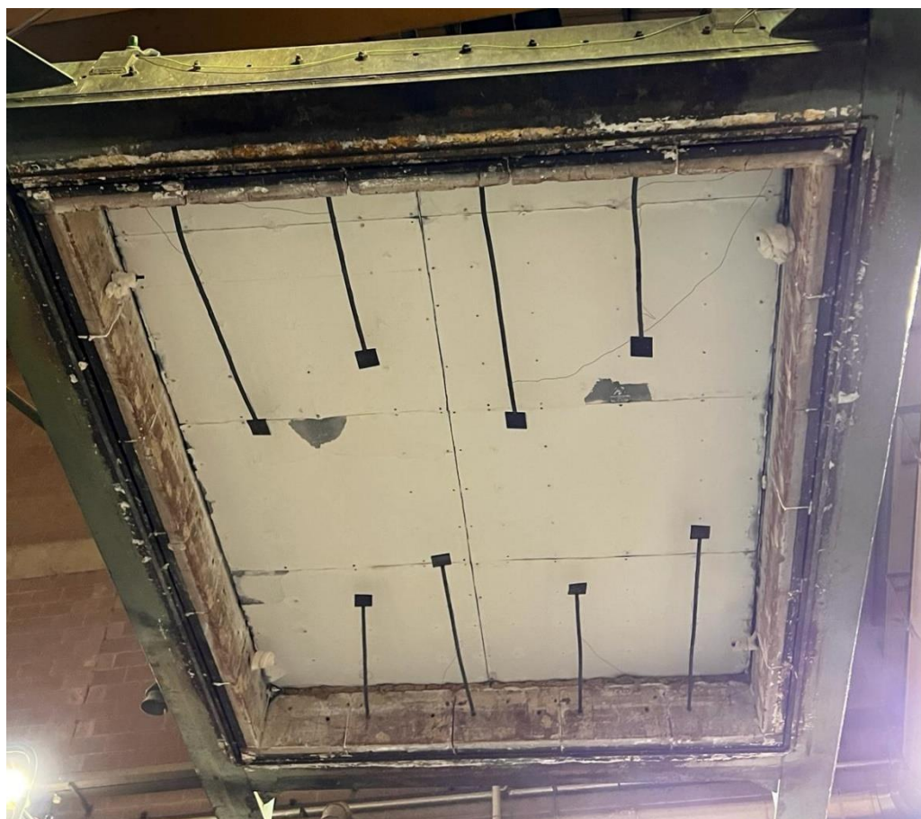
Photograph 18 - Detail of the exposed side of the sample after the test.
