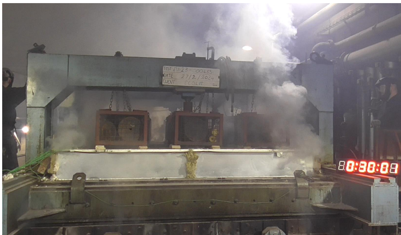
Photograph 11 - Detail of the unexposed side of the sample during the test. Photograph taken during minute 30.
