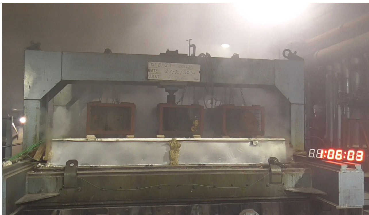
Photograph 17 - Overall view of the unexposed side of the sample at the end of the test.
